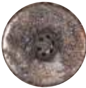
Injector before P.i. treatment.
