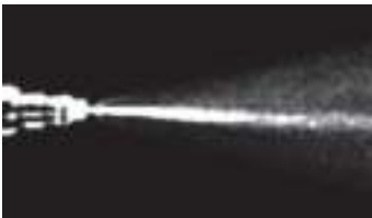
Injector spray pattern before P.i. treatment.
