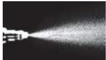
Injector spray pattern after P.i. treatment.
